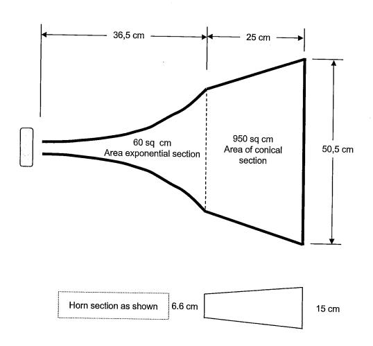
Weight of cast horn with compression driver installed, driver cover and fixing bolts is 12 kg
