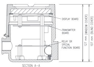
SECTION A-A WITHOUT SENSOR HEAD FITTED
